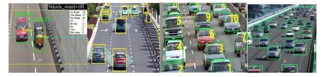
NableIT's AI-Based Vehicle Counting and Classification system is an advanced solution that leverages Artificial Intelligence and Deep Learning to count and classify vehicles accurately. This technology is crucial for traffic management, urban planning, and enhancing overall transportation efficiency.
